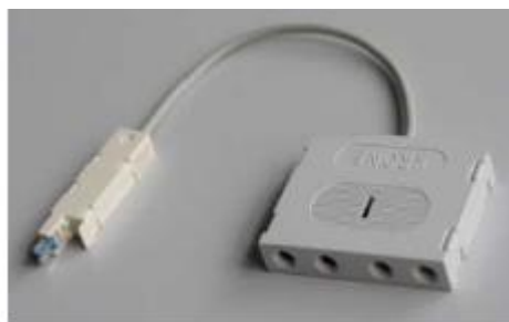
Figure 9: LSA-PLUS HD180 test cord, 4-pole [MID: 70142004-00]
