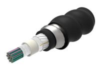
Fiber indoor/outdoor cable, Interlocking Armored, LSZH Riser-Rated, Gel-Free, Central Tube Rollable Ribbon, 432 fiber, Singlemode G.657.A2/B2, Feet jacket marking, Black jacket color, B2ca flame rating
