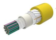
Fiber indoor cable, All-Dielectric, LSZH/Riser-Rated, Gel-Free, Central Tube Rollable Ribbon, 432 fiber, Singlemode G.657.A2/B2, Feet jacket marking, Yellow jacket color, Cca flame rating
