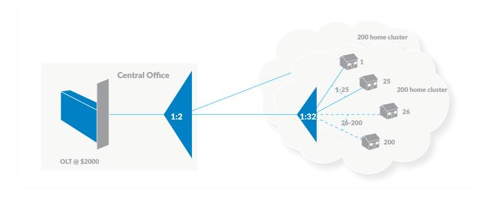
However this increased utilization rate must be considered along with the larger investment required in civil works and cable installation. The cluster sizes are larger and the distance between splitting point and end customer greater in centralized splitter architectures.
