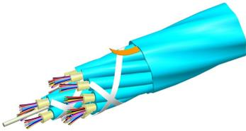
Fiber indoor cable, LazrSPEED® Plenum MPO Trunk, 64 fiber multi-unit with 8 fiber subunits, Multimode OM5, Gel-free, Feet jacket marking, Aqua jacket color
