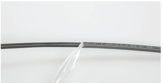
3.4.1 Remove outer jacket for 1.5 m leaving 25 cm of aramid strength member.
