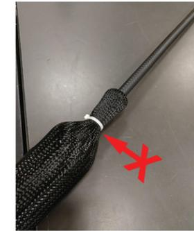
**d** Slide mesh in direction shown over cable end.
