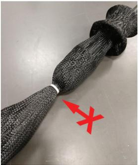
**f** Slide mesh in direction shown to uncover corrugated tube.
