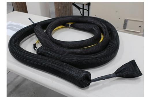
**4 Separate off lead end of cable assembly with pulling sock.**
