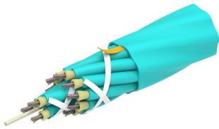
Fiber indoor cable, LazrSPEED® Low Smoke Zero Halogen Riser MPO Trunk Cable, 144 fiber with 24-fiber, 3.0mm subunits, Gel-free, Multimode OM4, Feet jacket marking, Aqua jacket color, B2ca flame rating
