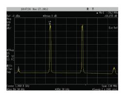
Defined as the unwanted signals generated by the non-linear mixing of two or more frequencies in a passive circuit, PIM is an obstacle to network efficiency.
