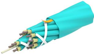
Fiber indoor cable, LazrSPEED® Plenum MPO Trunk Cable, 144 fiber with 24-fiber, 3.0mm subunits, Gel-free, Multimode OM4, Feet jacket marking, Aqua jacket color
