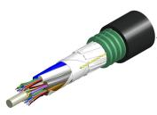
Fiber indoor/outdoor cable, LazrSPEED®, Mini Single Jacket/Single Armor, Riser/LSZH rated, 96 fiber, Gel-Filled, Stranded Loose Tube, Multimode OM3, Meters jacket marking, Black jacket color, Cca flame rating
