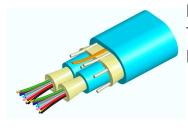
Fiber indoor cable, LazrSPEED® Low Smoke Zero Halogen Riser MPO Trunk, 16 fiber with 8 fiber 2.0mm subunits, Gel-free, Multimode OM4, Feet jacket marking, Aqua jacket color, Dca flame rating
