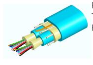
Fiber indoor cable, LazrSPEED® Low Smoke Zero Halogen Riser MPO Trunk, 16 fiber with 8 fiber 2.0mm subunits, Gel-free, Multimode OM5, Feet jacket marking, Aqua jacket color, Dca flame rating
