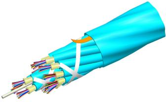
Fiber indoor cable, LazrSPEED® Low Smoke Zero Halogen Riser MPO Trunk, 72 fiber multi-unit with 8 fiber 2.0mm subunits, Gel-free, Multimode OM5, Feet jacket marking, Aqua jacket color, Dca flame rating
