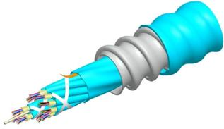
Fiber indoor cable, Plenum MPO Trunk, interlocking aluminum armored with plenum jacket, 36 fiber multi-unit with 12 Singlemode fiber subunits and 8 Multimode fiber subunits, Feet jacket marking, Aqua jacket color
