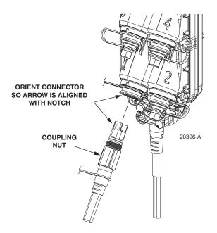
Figure 15. Connecting Drop Cable To MST Optical Port
