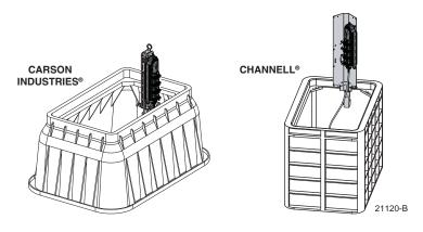
Figure 6. Typical Hand-Hole Mounting
