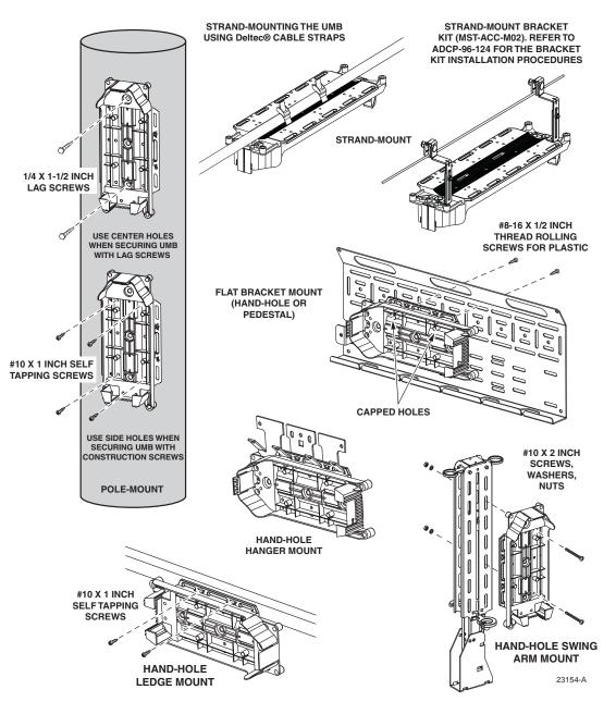
Figure 10. Installing the Universal Mounting Bracket (UMB)
