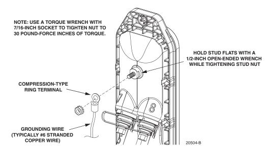
Figure 17. Grounding Lug Connection
