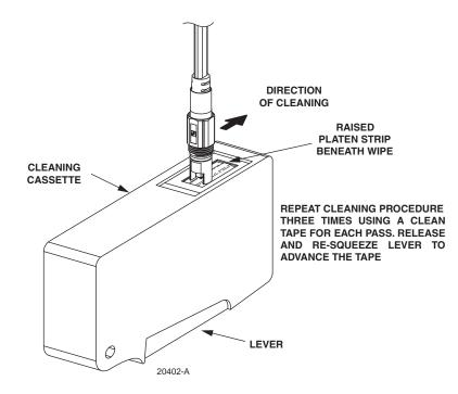
Figure 19. Cleaning Drop Cable Connector
