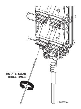
Figure 20. Cleaning Optical Port Connector and Adapter
