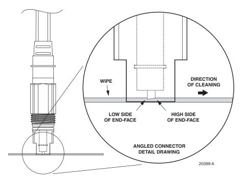
Figure 18. Angled Connector End-Face Detail
