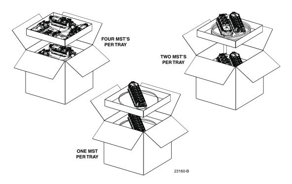
Figure 4. MST Cable Coiled and MST Placed in a Box
