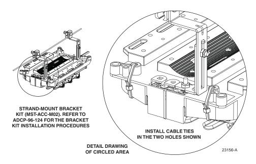
Figure 12. Securing Front of Strand-Mounted MST With Cable Ties
