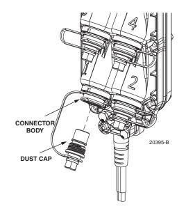
Figure 14. Optical Port Adapter Components
