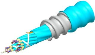
Fiber indoor cable, LazrSPEED® Plenum MPO Trunk, interlocking aluminum armored with plenum jacket, 12 fiber, Gel-free, Multimode OM4, Feet jacket marking, Aqua jacket color
