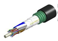
Fiber OSP cable, TeraSPEED® Mini Single Jacket/Single Armor, 12 fiber, Gel-Filled, Stranded Loose Tube, Singlemode G.652.D and G.657.A1, Meters jacket marking, Black jacket color
