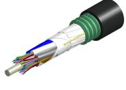
Fiber OSP cable, TeraSPEED® Mini Single Jacket All-Dielectric, 72 fiber, Gel-Filled, Stranded Loose Tube, Singlemode G.652.D and G.657.A1, Meters jacket marking, Black jacket color
