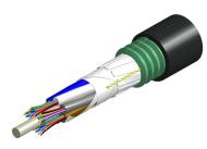
Fiber OSP cable, TeraSPEED® Mini Single Jacket All-Dielectric, 72 fiber, Gel-Filled, Stranded Loose Tube, Singlemode G.652.D and G.657.Al, Meters jacket marking, Black jacket color
