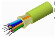
Fiber indoor cable, LazrSPEED® Low Smoke Zero Halogen Riser Distribution, 6 fiber single-unit, Multimode OM4, Feet jacket marking, Aqua jacket color, B2ca flame rating
