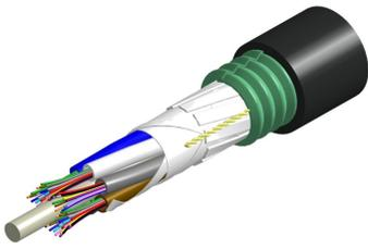
Fiber indoor/outdoor cable, LazrSPEED®, Single Jacket/Single Armor, Low Smoke Zero Halogen (LSZH), 144 fiber, Multimode OM4, Gel Filled , Stranded Loose Tube, Black jacket color, Meters jacket marking, Cca flame rating
