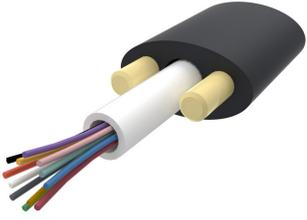
Fiber drop cable, Self-Supporting All-Dielectric, 12 fiber Arid Core construction, central loose tube, Gel-filled, Singlemode G.657.A2/B2, Feet jacket marking, Black jacket color, Build America Buy America (BABA)
