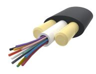
Fiber outdoor drop cable, LightScope ZWP® Self-Supporting All-Dielectric, Singlemode G.652.D and G.657.Al, 2 fiber Arid Core construction, Gel-filled, central loose tube, no ripcords, Feet jacket marking, Black jacket color
