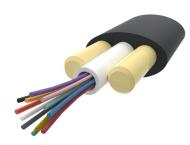
Fiber outdoor drop cable, LightScope® ZWP Self-Supporting All-Dielectric, Singlemode G.652.D and G.657.A1, 4 fiber Arid Core construction, Gel-filled, central loose tube, no ripcords, Feet jacket marking, Black jacket color
