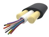
Fiber outdoor drop cable, LightScope® ZWP Self-Supporting All-Dielectric, Singlemode G.652.D and G.657.Al, 6 fiber Arid Core construction, Gel-filled, central loose tube, no ripcords, Feet jacket marking, Black jacket color
