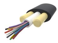
Fiber outdoor drop cable, LightScope® ZWP Self-Supporting All-Dielectric, Singlemode G.652.D and G.657.A1, 12 fiber Arid Core construction, Gel-filled, central loose tube, no ripcords, Feet jacket marking, Black jacket color
