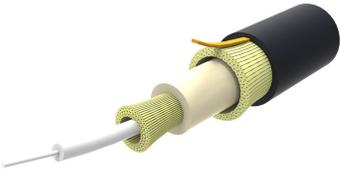
Fiber indoor/outdoor drop cable, All-Dielectric, 1 fiber Tight Buffer construction, riser, drop all-dielectric, Singlemode G.657.A2/B2, Gel-free, Feet jacket marking, Black jacket color
