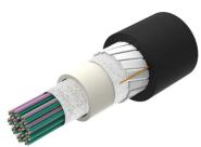
Fiber OSP cable, Non-Armored, All-Dielectric, Arid-Core, Dry Central Tube Rollable Ribbon, 288 fiber, Singlemode G.652.D and G.657.A1, Gel-free, Feet jacket marking, Black jacket color
