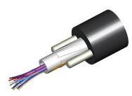
Fiber indoor/outdoor cable, LightScope® ZWP Single Jacket All-Dielectric, Singlemode G.652.D and G.657.Al, 12 fiber Arid Core construction, Gel-filled, central loose tube, Meters jacket marking, Black jacket color
