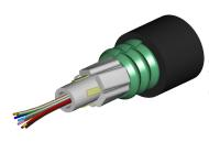
Fiber drop cable, LightScope® ZWP Single Jacket Single Armor Outdoor Drop Cable, 12 fiber Arid Core construction, central loose tube, Gel-filled, Singlemode G.652.D and G.657.A1, Custom jacket marking, Black jacket color
