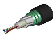
Fiber drop cable, LightScope® ZWP Single Jacket Single Armor Outdoor Drop Cable, 8 fiber Arid Core construction, central loose tube, Gel-filled, Singlemode G.652.D and G.657.Al, Meter jacket marking, Black jacket color
