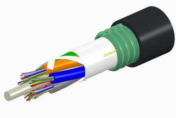
Fiber OSP cable, LightScope® ZWP Single Jacket/Single Armor, 72 fiber, Gel-Free, Stranded Loose Tube, Singlemode G.652.D and G.657.A1, Meters jacket marking, Black jacket color
