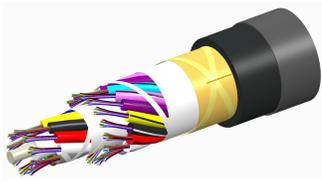
Fiber indoor/outdoor cable, LightScope® ZWP, Single Jacket All-Dielectric, Riser Rated, 12 fiber, Gel-Free, Stranded Loose Tube, Singlemode G.652.D and G.657.A1, Meters jacket marking, Black jacket color
