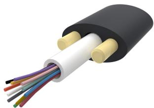
Fiber outdoor drop cable, LightScope® ZWP Self-Supporting All-Dielectric, Singlemode G.652.D and G.657.A1, 8 fiber Arid Core construction, Gel-filled, central loose tube, Feet jacket marking, Black jacket color
