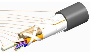
Strength Elements Binder Water Swellable Tape Ripcord (1) Binder 2.5 mm Gel-Free Buffer Tubes 250 micron Fibers **Dielectric Strength Member**
