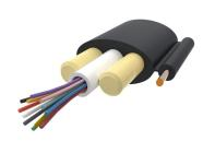
Fiber Hybrid drop cable, LightScope® ZWP Fiber + Tone Wire Outdoor, 2 fiber Arid Core construction, central loose tube, Gel-filled, Singlemode G. 652.D and G.657.A1, Feet jacket marking, Black jacket color
