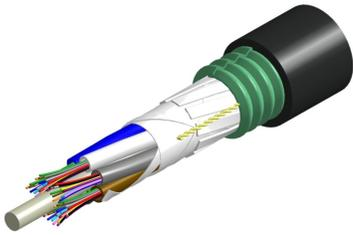
Fiber OSP cable, LightScope ZWP® Mini Single Jacket/Single Armor, 24 fiber, Gel-Filled, Stranded Loose Tube, Singlemode G.652.D and G.657.A1, Meter jacket marking, Black jacket color
