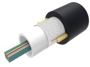
Fiber OSP cable, Non-Armored, All-Dielectric, Gel-Filled Central Tube Ribbon, 36 fiber, Singlemode G.652.D and G.657.A1, Feet jacket marking, Black jacket color
