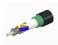
Fiber indoor/outdoor cable, TeraSPEED®, Single Jacket/Single Armor, Low Smoke Zero Halogen (LSZH), Singlemode G.652.D and G.657.A1, 6 fiber, Gel Filled, Stranded Loose Tube, Meters jacket marking, Black jacket color, B2ca flame rating
