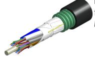
Fiber OSP cable, LightScope® ZWP Mini Single Jacket/Single Armor, 96 fiber, Gel-Filled, Stranded Loose Tube, Singlemode G.652.D and G.657.A1, Meters jacket marking, Black jacket color
