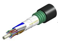
Fiber OSP cable, LightScope® ZWP Mini Single Jacket/Single Armor, 72 fiber, Gel-Filled, Stranded Loose Tube, Singlemode G.657.A2, Meters jacket marking, Black jacket color
