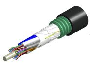
Fiber OSP cable, LightScope® ZWP Mini Single Jacket/Single Armor, 96 fiber, Gel-Filled, Stranded Loose Tube, Singlemode G.657.A2, Meters jacket marking, Black jacket color
