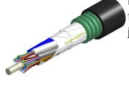
Fiber OSP cable, LightScope® ZWP Mini Single Jacket/Single Armor, 144 fiber, Gel-Filled, Stranded Loose Tube, Singlemode G.657.A2, Meters jacket marking, Black jacket color
