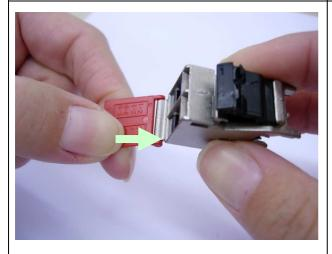
Check both sides are fully inserted and the dust cover is functional and rotates.
