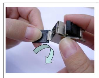
For disassembling the existing dust cover, pivot it while turning it toward the bottom.
