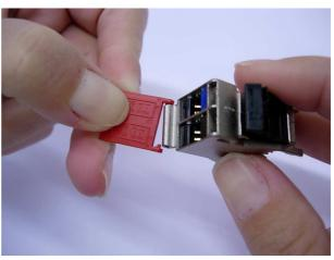
Take the new one. For assembling the new dust cover, place one side into the hinge and pivot the other side while pushing.
