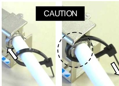
Locate the cable tie as shown and tighten, pressing the braid to the rear housing.
