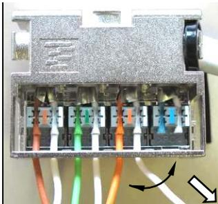
Extract the group from the Pistol Tool and remove the cut wires, keeping the SEC into the housing.
