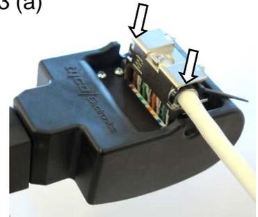
Insert the assembly into the Pistol Grip Tool, up to the limit, and terminate wires.
