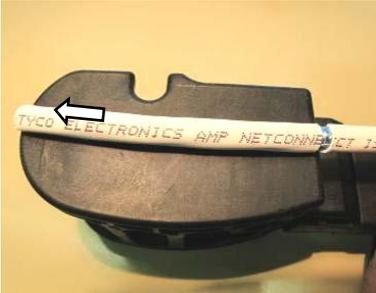
Remove 70-80mm of cable jacket and fold the braiding back along the outer jacket, fixing the drawing wire when necessary.
