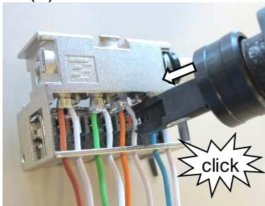
Alternatively to the Pistol Grip Tool, or for re-termination, the Impact Tool can be used on every wire.
