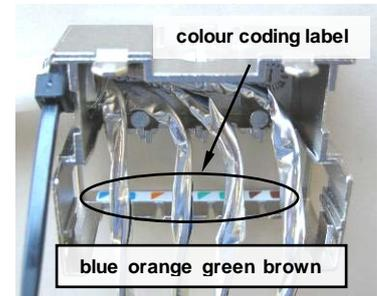
Sort the pairs inside the rear housing according to the colour coding label.
