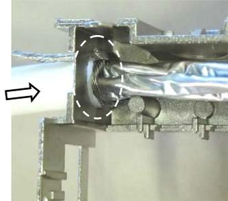
Pass the cable through the cable exit until the cable jacket is inside the housing.
