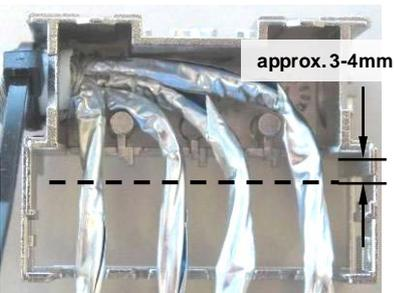
Mark the foils using the rear housing reference, as shown.
