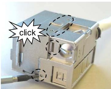
If necessary, use a flat-blade screwdriver to gently open AMP CO Ultra Housing.
