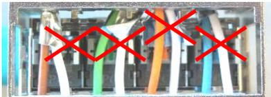
Check carefully the correct position of the wires over the SEC IDC blocks (re-arrange the wires if necessary) and the correct position of each pair's foil: wrapped around the wires and as close as possible to the IDC block (without touching).
