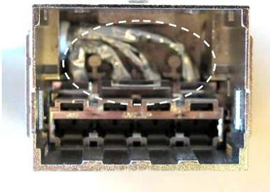
Foils contact to SEC and correct pairs distribution.
