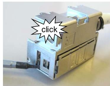
If necessary, use a flat-blade screwdriver to gently open SEC.
