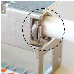
Wrap the twisted braid once around the fixing feature, as shown.
