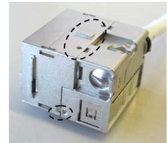
Top and lateral pins inserted into their cavities.
