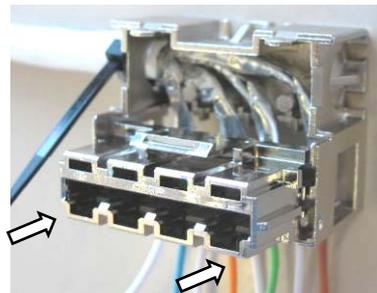
Insert the SEC into rear housing, positioned as shown, up to the limit.
