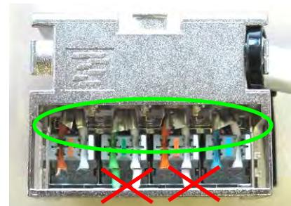
Check there are no cut-wire fragments left and re-check the correct position of the foils.
