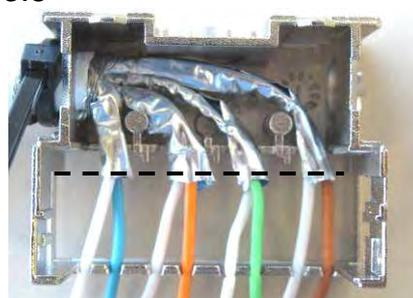
Cut-out the foils and locate each pair in the correct slot.
