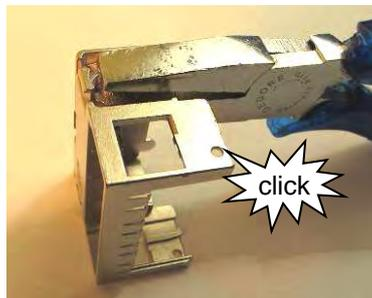
Use pliers to break-out the desired cable exit ("top" "right" or "left") from the rear housing.
