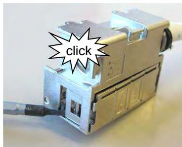
If necessary, use a flat-blade screwdriver to gently open SEC.
