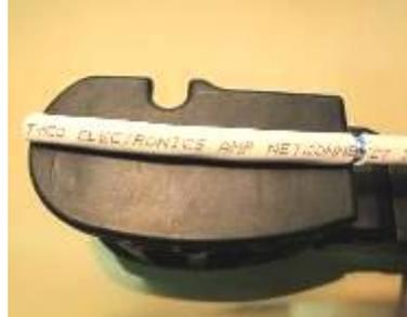
Remove approx. 70mm of cable jacket and fold the braiding back along the outer jacket, fixing the drain wire when necessary.
