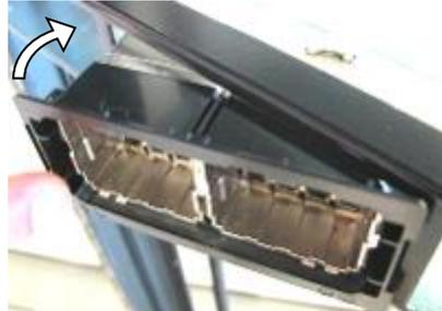
Take the Quick-Fit Body assembly with AMP CO Ultra already assembled in and place it into the side rib of the panel. Pivot the opposite end while pushing it towards the side to allow the side latch of the Body to enter into the panel.
