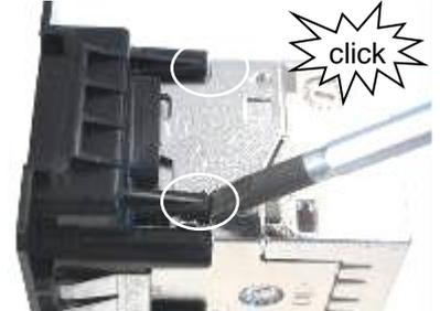
Remove the AMP CO Ultra housing from Quick-Fit Body by means of unlocking the 4 latches.
