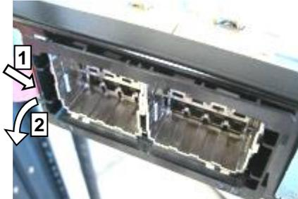
Unlock the Quick-Fit Body from panel opening by means of pushing latch (1) and rotating Quick-Fit Body (2).
