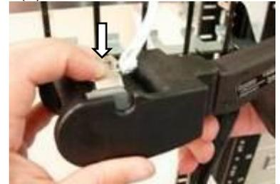
Insert the assembly into the Pistol Grip Tool, up to the limit, and terminate the wires.
