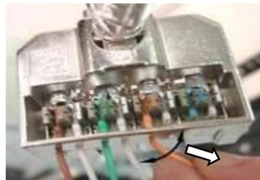
Extract the group from the Pistol Tool and remove the cut wires, keeping the SEC position into the housing.
