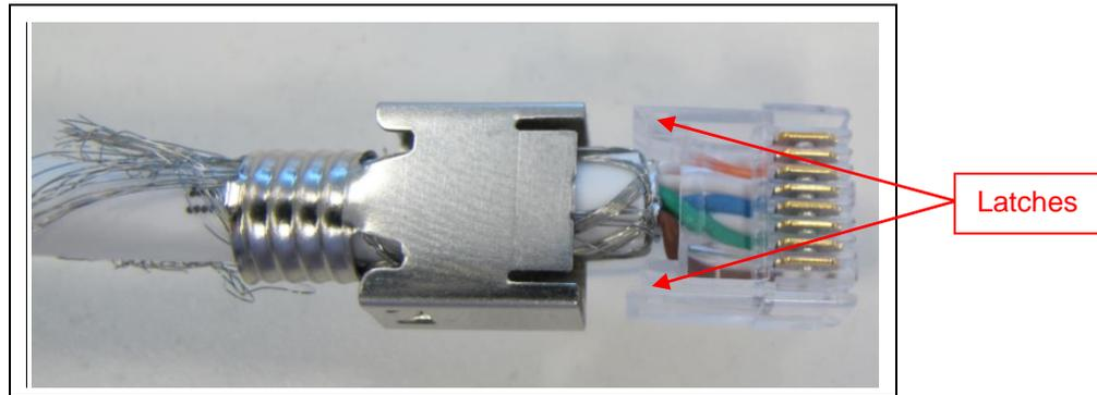
**Figure 10. Secure Wire Holder into Housing**
