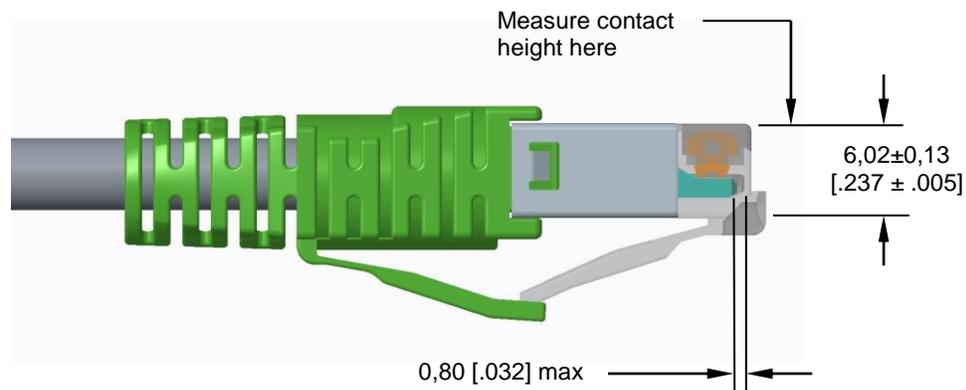
Figure 16. Plug Tolerances
