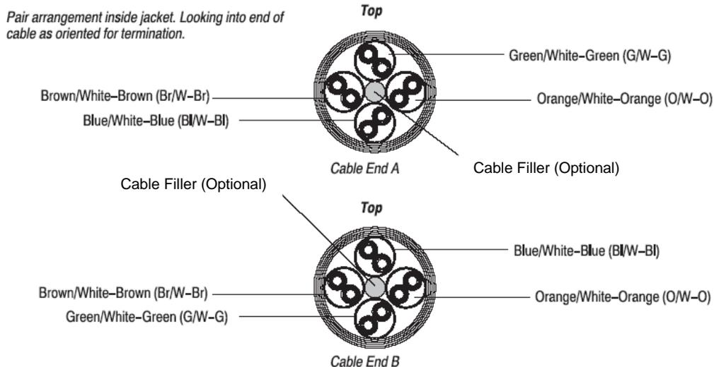
**Figure 2. Arrangement of Color-Coded Pairs**
