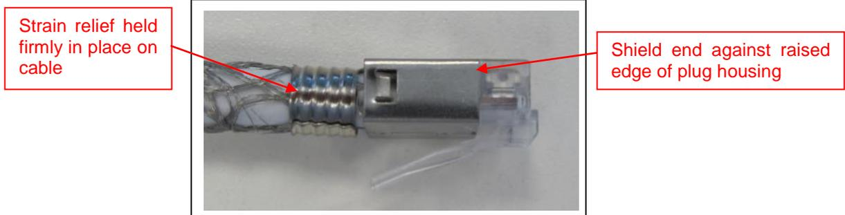
**Figure 13. Shield Against Raised End of Housing**
