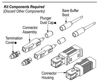
Connector kit is shipped with these installed onto connector assemblies. Keep them in place until ready for assembly.
