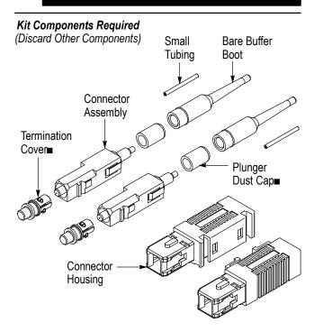
Connector kit is shipped with these installed onto connector assemblies. Keep them in place until ready for assembly.
