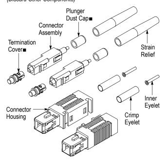
■ Connector kit is shipped with these installed onto connector assemblies. Keep them in place until ready for assembly.
