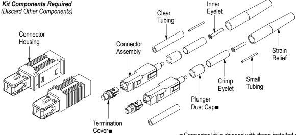
■ Connector kit is shipped with these installed onto connector assemblies. Keep them in place until ready for assembly.
